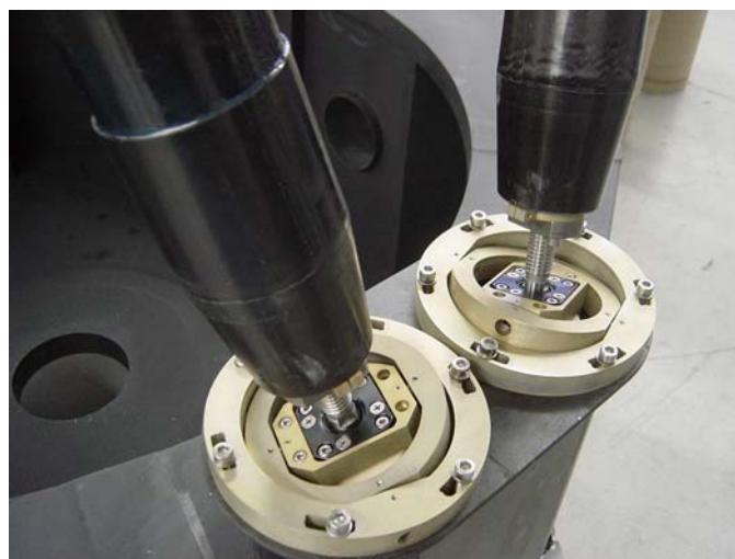
Figure 3: Lower strut mount. Drive motor located under mount
