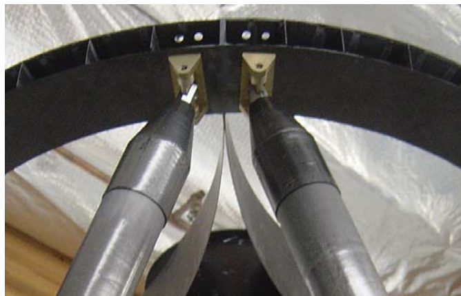
Figure 2: Strut tube top mounting to head ring with flex pivot Gimbal.
