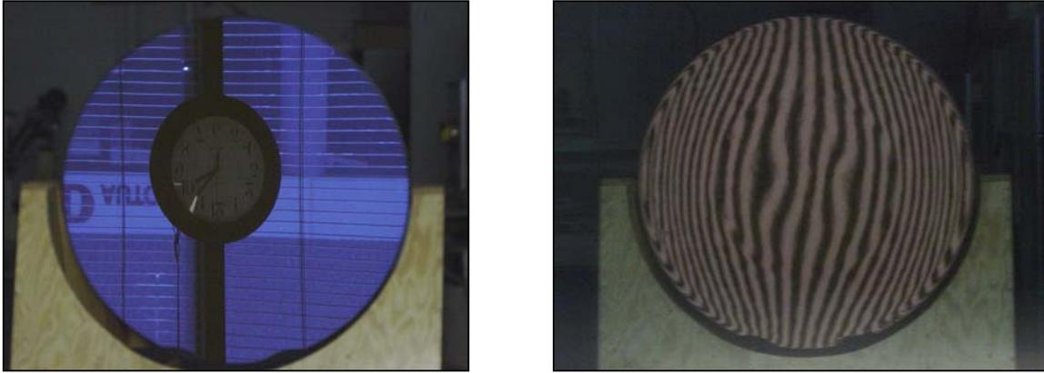
**Figure 11.** LEFT, image shows the 1m parabolic mirror in the test stand and RIGHT, 50 lines per in Ronchigrams of the 1m before final figuring of the 1m mandrel. Fringes are smooth despite astigmatism in the mirror from its being supported on the bottom edge without core reinforcement. Mirror weighs 18 kg.
