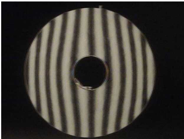
Figure 7. Image shows a 50 lines per inch Ronchigram of a CFRP Cassegrain mirror, exhibiting the same paraboloidal shape as in the figure above. This mirror was produced for the NRL's 40cm Adaptive Optics telescope and will be ready for delivery by May 2006.
