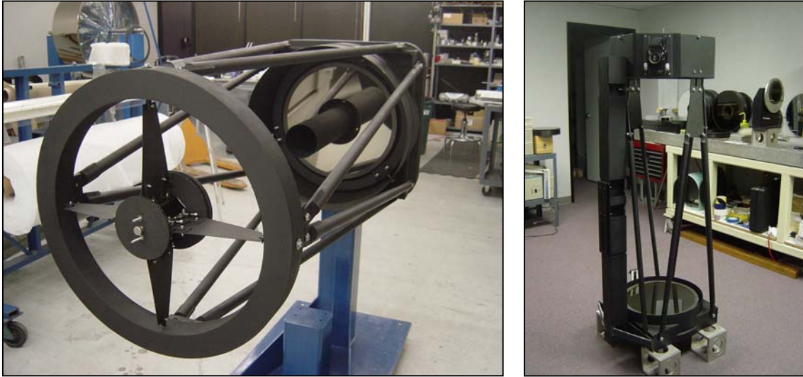
Figure 3. LEFT, NRL's Cassegrain 40cm, All-CFRP composite telescope, weighs 10 kg complete with optics, RIGHT Newtonian 40cm all-CFRP composite telescope for astronomical image testing, weighs 8 kg complete with optics.
