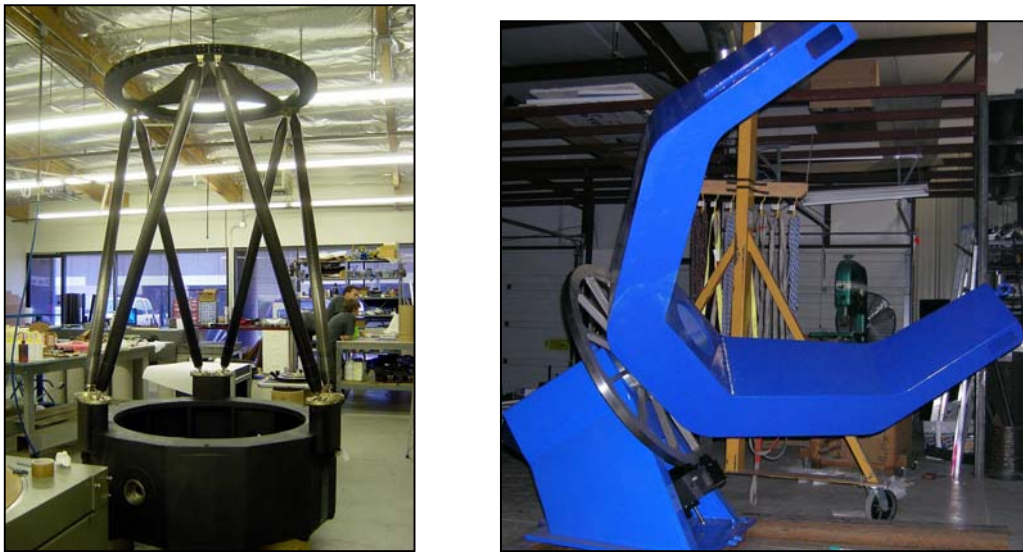
Figure 12. LEFT, image shows the All CFRP 1m ULTRA telescope, weighs 61 kg without optics. The secondary mirror is controlled in 6 axis by a piezo driven hexapod actuation system. The head ring, struts upper “U”-joints and secondary mirror have a combined mass of 11.5kg. RIGHT ACE’s polar mount for ULTRA.
