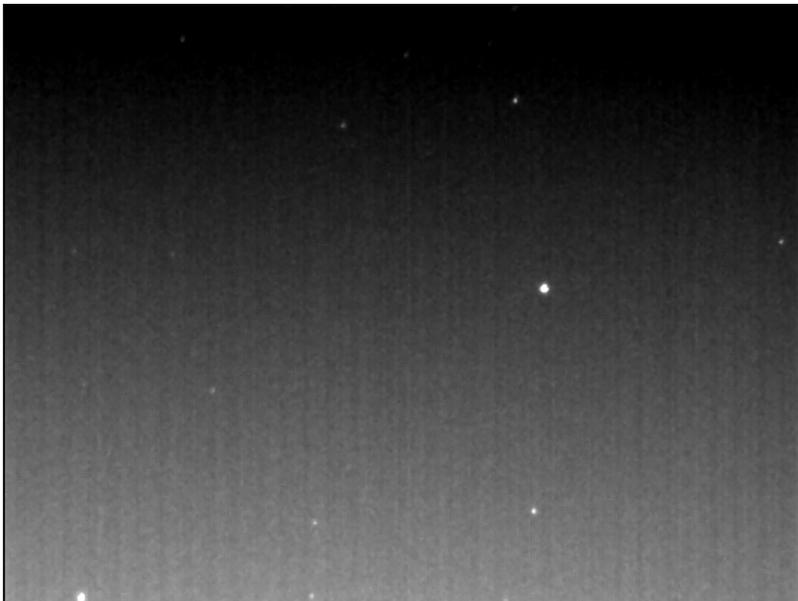
**Figure 10.** Image of Polaris, April 2006, 0.05 sec exposure, no filter. The image subtend an angle of roughly 3 to 4 arcseconds. The smaller stars subtend as low as 2 arcseconds. The seeing was not likely to be better than 2 arcseconds, implying that the images were mostly seeing limited or limited by tracking errors relating to the mount.
