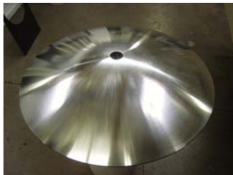
Figure 5. CFRP 0.75m diameter secondary mirror (built at CMA) for ALMA telescopes.
