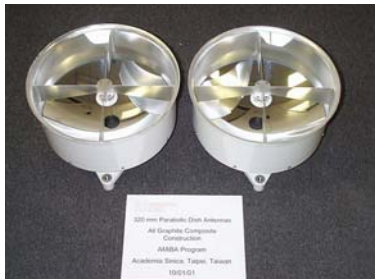
Figure 6. Two CFRP 320mm diameter Cassegrain systems built at CMA for the ASIAA AMiBA experiment on Mauna Loa, HI.
