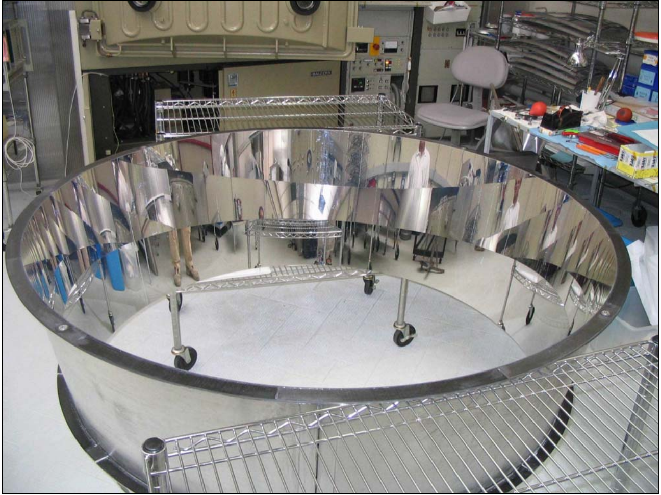
Figure 10. FM (upside down) after Aluminum +SiO over coating at ZOAT, IT. The mirror was coated on the outside surface as well for environmental resistance.
