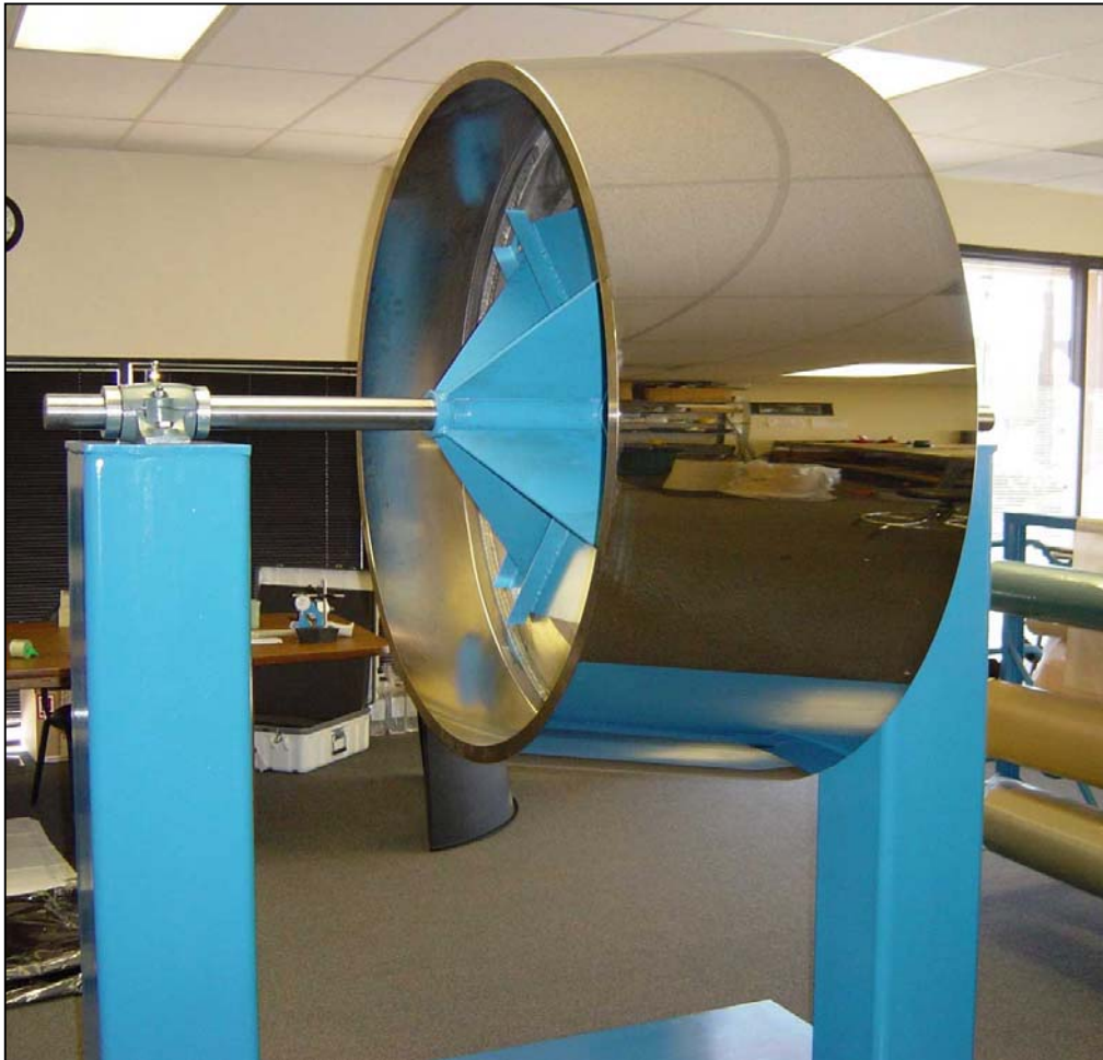
Figure 4. Nickel coated aluminum mandrel for the RICH mirror. The mandrel is shown on a rotating holding fixture.
