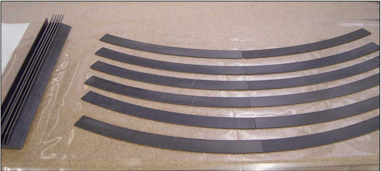
Figure 6. Image shows the CFRP flange arc sections and the vertical “L” brackets
