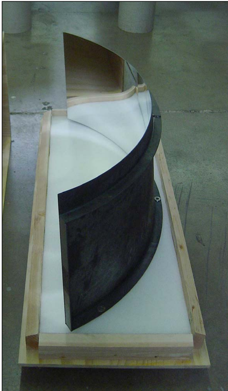
Figure 5. Prototype RICH Mirror, EM readied for shipment to Milan, IT. The EM is shown with aluminum coating and ribs and flange structure to help maintain figure during testing and evaluation by CGS.
