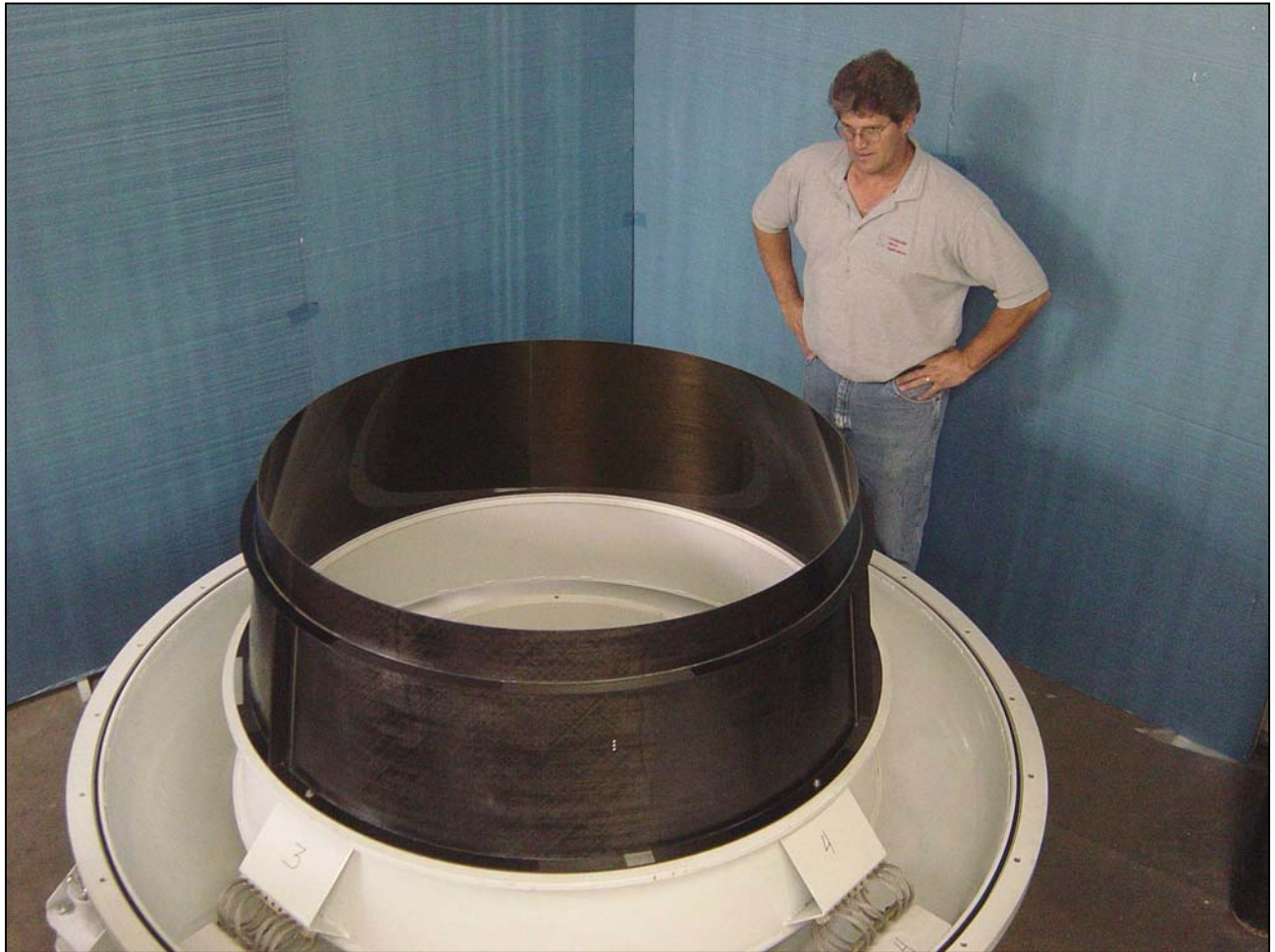
Figure 9. Image of the FM on the container mount, shown are the upper and lower flanges and vertical ribs in place.
