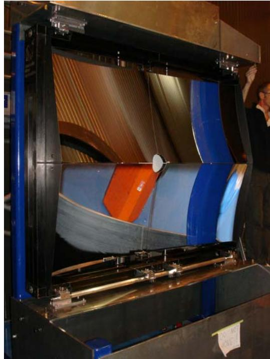
Figure 6. Photos of the coated RICH1-CMA mirrors. Left; coated mirror at SESO. Right, the 4 coated mirrors assembled in the carbon fiber onto the alignment rig at CERN in July 2007.
