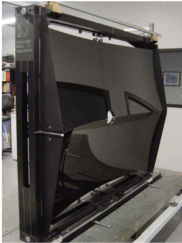
Figure 4. The final mirrors and frame assembly after alignment at CMA
