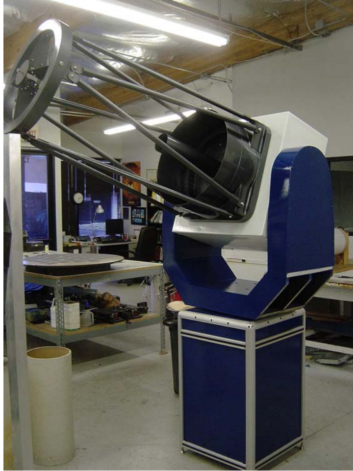
Figure 3- Lightweight telescope (in black) mounted on portable AO system (white) and lightweight mount (blue fork).
