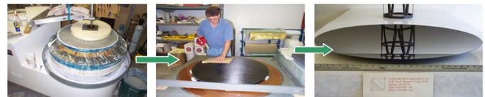
*Figure 2. The CFRP fabrication sequence appears from left to right: processing the glass mandrel; lay-up of CFRP over the glass mandrel; and release CFRP mirror from the mandrel, ready for coating without additional figuring or polishing.*
