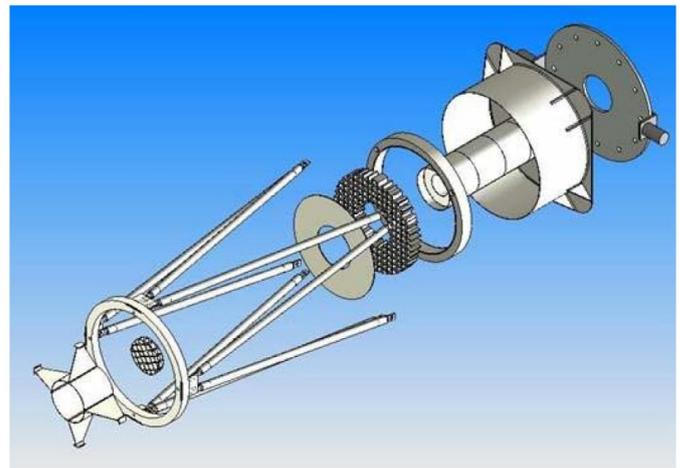
*Figure 1. This exploded view of the CFRP telescope shows the position of the composite optics.*
