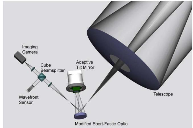
**Figure 4.** The adaptive optics system shown here is used for the lightweight telescope.
