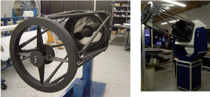
**Figure 3.** The 40cm, all-CFRP composite telescope weighs 10 kg complete with optics (left). The telescope installed on its mount is shown on the right.
